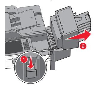
**2** Open the finisher door, and then removed the jammed paper.
